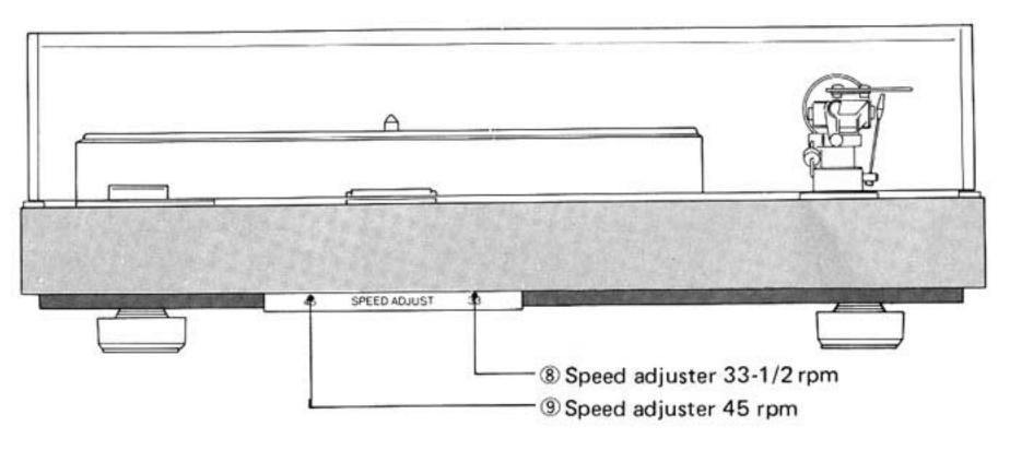
of the adjuster increases rotation speed, while it is decreased with a counter-clockwise turn. When the stroboscope pattern appears to be stationary, correct rotation speed has been obtained. Before making this adjustment, be sure to check the mains line frequency, i.e., 60Hz or 50Hz.
