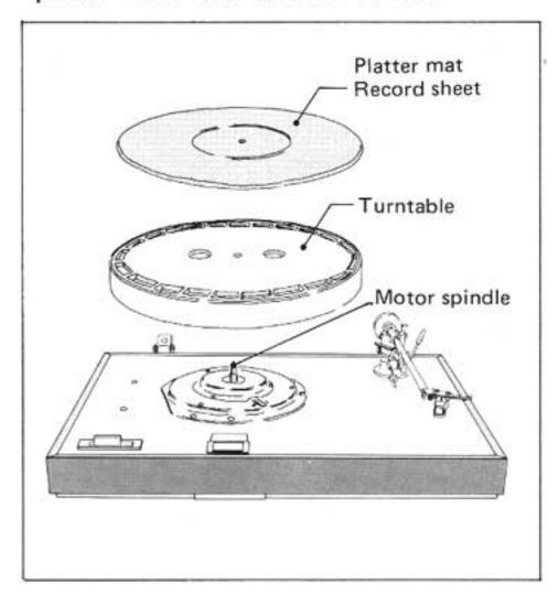
bottom of the packing case. After having taken off the mat from the platter, insert carefully the platter in the center shaft of the motor, holding it by fingers through the 2 holes. Now turn the platter manually to check if correct setting-up is obtained. Then put the mat on the platter.
