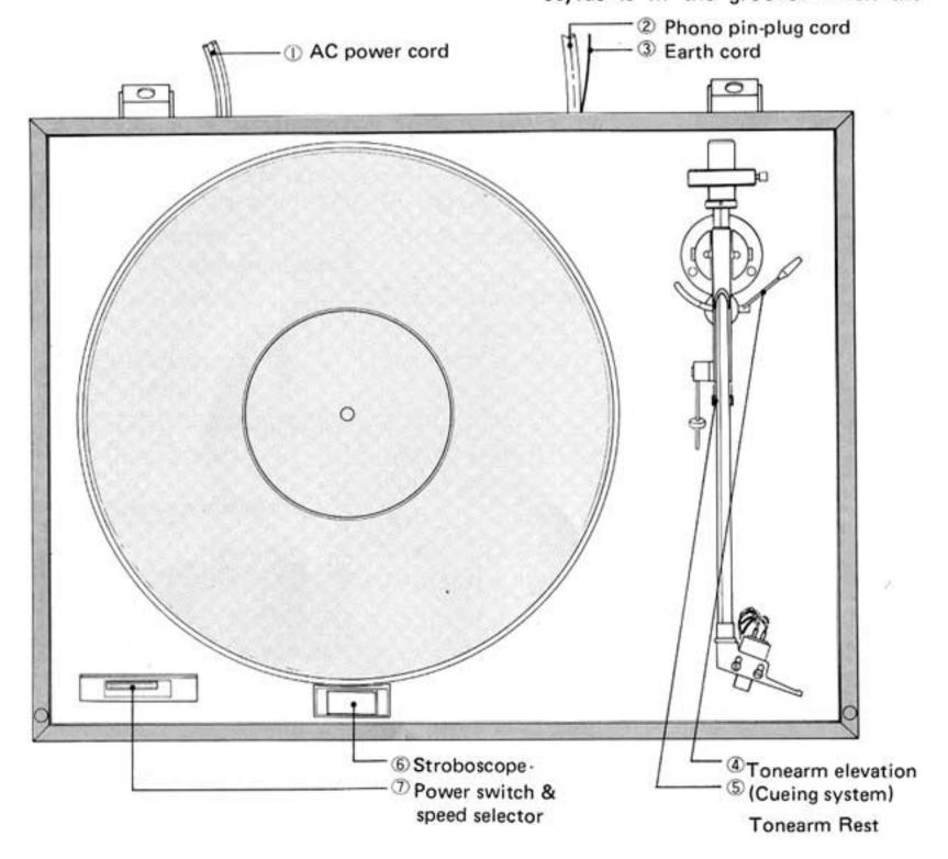
lever is lifted up, the tonearm will gently come up from the surface. Now it is possible to reset the tonearm at the arm-rest without damaging the disc.
